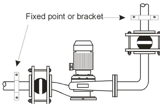
Rubber bellows will exert a pressure thrust in service and must be anchored to protect adjacent pipework and equipment. Rubber bellows will extend under pressure and must be anchored to prevent this happening.
