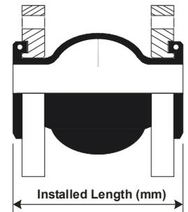
**Installation** Rubber bellows should be installed at their neutral (supplied) length. Confirm that the gap left between the mating flanges in the pipework corresponds exactly with the neutral (supplied) length of the rubber bellows. Pipework should be true and straight. Any adjustments should be made to the pipework before the rubber bellows are fitted. See appropriate Stourflex data sheets for the installation length of the rubber bellows being installed.
