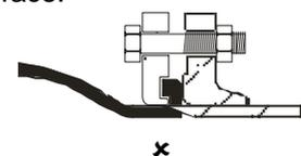
Flange bolts must not be over tightened, bolts should be tightened gradually and evenly and in a crosswise manner. Bolts should be positioned so that the bolt head is nearest the bellows to prevent the bolt damaging the bellow in service. Tightness of bolts should be checked approximately seven days after installation.
