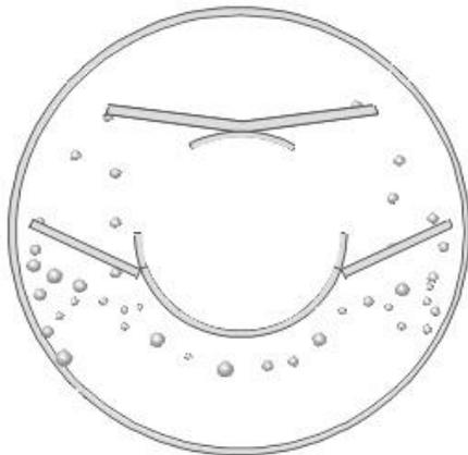
As the water reaches the bottom chamber the velocity is reduced even further and a turbulence free area is created.
