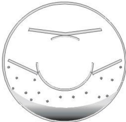
The still turbulence free area created allows solid particles heavier than water to settle and be collected in the bottom of the adjoining dirt chamber and remain undisturbed until drained manually. Large air bubbles will be removed quickly. Micro bubbles and solid particles will be removed over a period of time.
