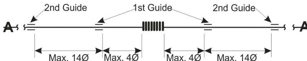
Typical pipework example showing installation where a Stourflex Axial Expansion joint is installed with JP150 Expansion Joint guides and JP175 Suspended Pipe Anchors.
