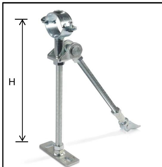
A centre line dimension H+ of 350mm should not be exceeded when using M16 angular braces
