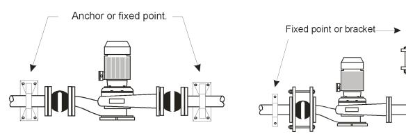
Rubber bellows will exert a pressure thrust in service and must be anchored to protect adjacent pipework and equipment. Rubber bellows will extend under pressure and must be anchored to prevent this happening.
